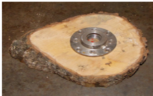
End-grain blank with a faceplate (maple)
