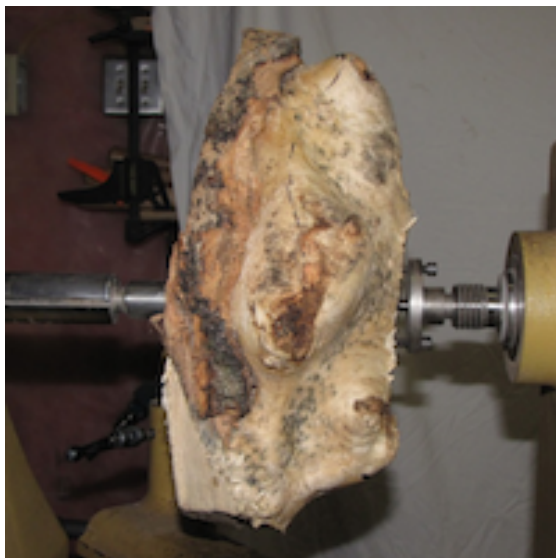
Two views of an aspen burl mounted on a lathe using an Elio drive and a rotating tail stock
