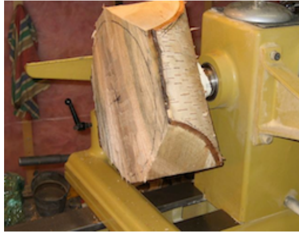
A birch bowl blank mounted with a faceplate
