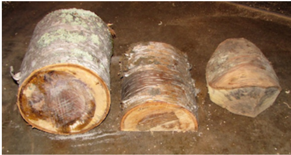
A round birch log shown whole, split, and cut into a boat-shaped bowl blank
